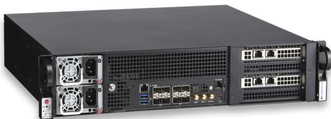
SYS-212D-72C High Core Count RAN DU Platform
